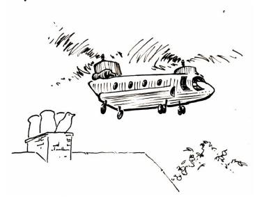
Chinook Helicopter – can carry 10 tonnes and can reach 200 mph. The body is 15 metres long, holds 4,000 litres of fuel, and two turbines generate about 5,000 horse power. It uses 1.2 tonnes of fuel an hour.
