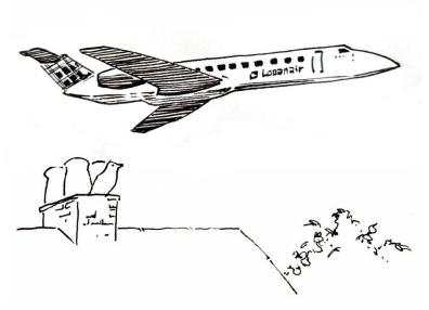
This is a Loganair Embraer ERJ-145. Embraer is a Brazilian company that uses parts from all over Europe to build planes Its maximum speed is 520mph, range is about 2300 miles – Exeter to Tunisia. The aircraft weighs around 13 tonnes.
